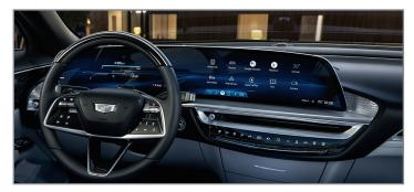
**ON DISPLAY** A LYRIQ driver can access a range of information projecting from a 33-inch curved LED display that covers most of the vehicle's dashboard. The display divides into three sections, covering (left to right) trip information, instrument gauges and the infotainment system.
